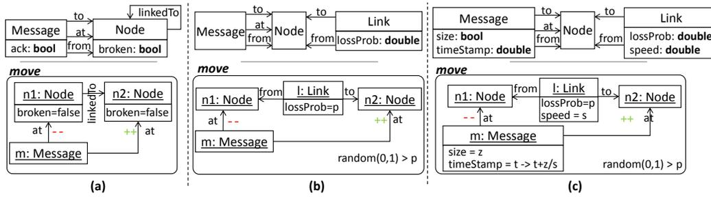
Figure 1: Three network language variants, and one example rule of each. (a) Simple links with node failures and acks. (b) Rich links with communication failures. (c) Rich links with communication failures and time. Rules use a compact notation with ++ denoting element creation, -- element deletion, and -> attribute change.
