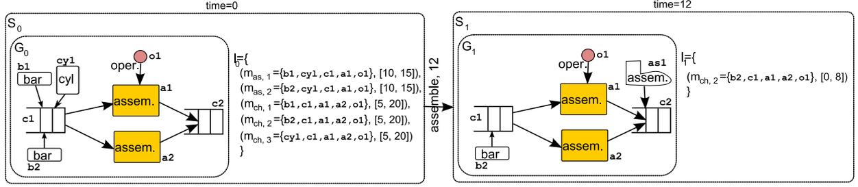
Fig. 21. One Step in a Timed Rule-Based Simulation.
