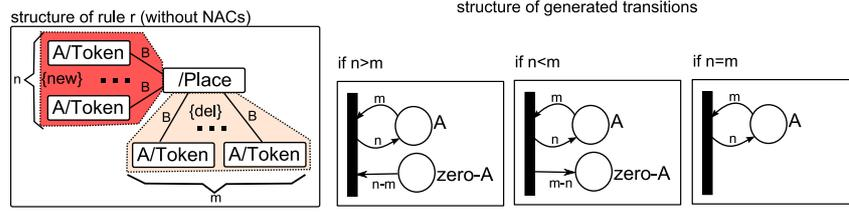
Fig. 30. Simplification of Weight for Zero-Testing Places.
